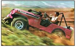
Starting in 1976, the CJ-7 was released to the public. It was 10 inch longer version of the CJ-5 with noticeably larger door openings without the reverse curve openings of the CJ-5. It featured a wider rear chassis section and rear suspension set wider on the axles for better stability. The CJ-7 offered for the first time an optional fiberglass hardtop and factory steel doors. Between 1976 and 1986 over 379,000 were produced.
