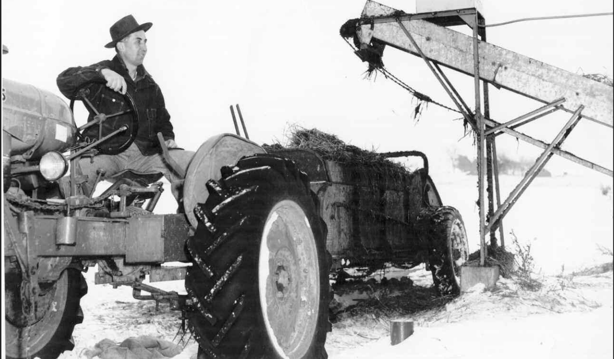
Lester (41 years old) is showing Roger (8 years old) how the new Jamesway barn cleaner operates. “Saves my back and cuts chore time in half,” is what Lester Hermanson siad of his Jamesway cleaner. The year was 1953. Photos indicate how the cleaner works inside the barn and conveys outside to the manure spreader. (Submitted by Roger Hermanson)
