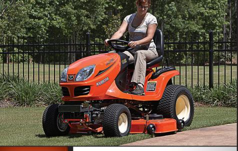
GR SERIES: **GLIDE STEER**  Classic garden tractor style with exclusive Glide Steer technology. power steering, all-wheel traction and 20 HP gas or 21 HP diesel Kubota engine.
