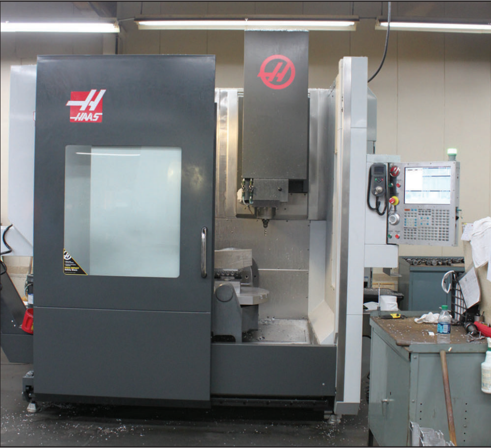
THESE TWO MACHINES were purchased recently by Lyons manufacturing. The machine above is a Hwacheon Cutex-240 turning center. This machine is equipped with two spindles and is capable of machining a complete part in one operation. This machine is used for turning titanium bolts used on the Boeing 777. At the left is a Haas UMC-750 machining center. This machine is equipped with a 12,000 RPM, 30 HP spindle. This machine is used for high speed 5-axis machining of complex aircraft parts for the Boeing 737 & 787.
