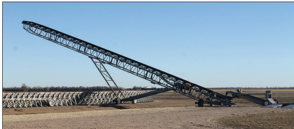
The new MKC grain bunker includes a large motorized grain conveyor belt. The conveyor belt can be moved as needed.
