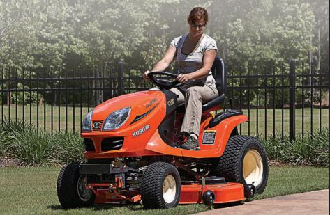
GR SERIES: GLIDE STEER Classic garden tractor style with exclusive Glide Steer technology, power steering, all-wheel traction and 20.5 HP\*\* gas or 21 HP\*\* diesel Kubota engine.
