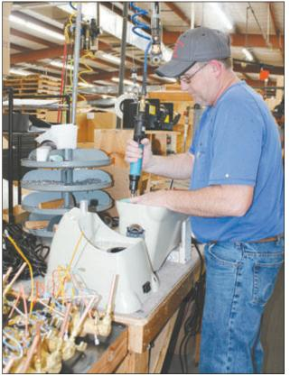
**HELPFUL TOOLS** — Twenty-eight-year Jiffy Steamer employee Bryan Cranford of Hornbeak used a semi-automated screwdriver to install a metal base on a steamer being assembled at the local business, which celebrates its 77th anniversary this year. The company installed the semi-automated equipment to help employees who once had to tighten screws by hand. The equipment helps reduce repetitive motion injuries.
