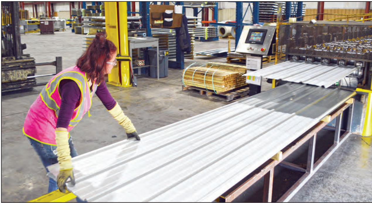
Union Corrugating employee Danielle Moore operates a roll former that’s producing the company’s most popular item, a residential/ agriculture panel. The panel is typically manufactured in 26 or 29 gauge.
