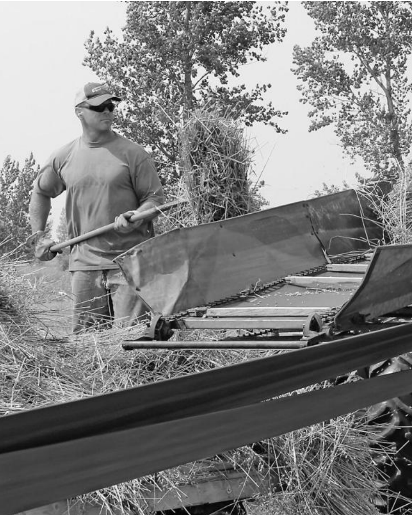
Jim Sobotzak loads up the bales into the threshing machine, which, in this instance, is powered by a belt pulley attached to an older model John Deere tractor.
