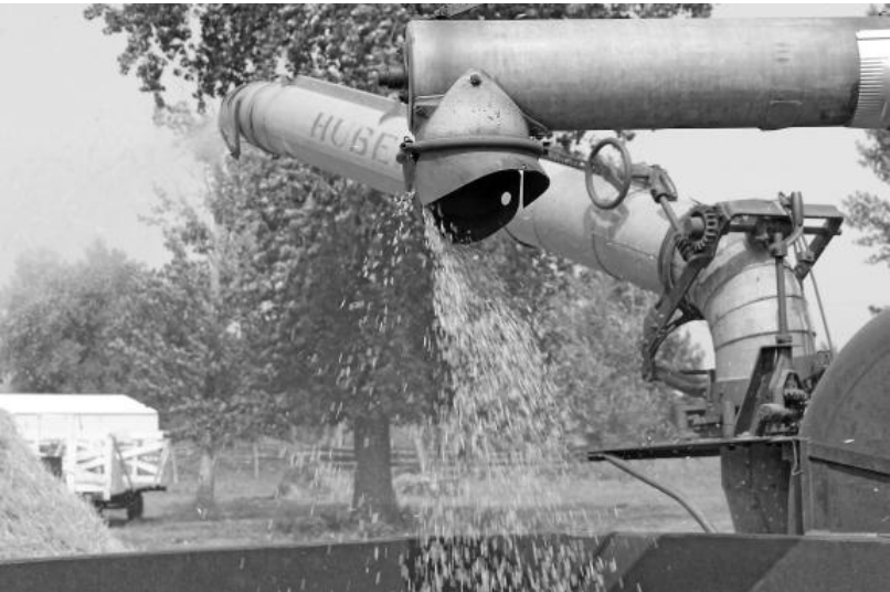
In the last stage of the threshing process, the separated oats are gathered while the straw is blown into a pile.
