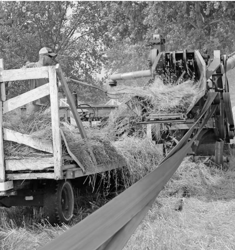
Jim Sobotzak loads up the bales into the threshing machine, which, in this instance, is powered by a belt pulley attached to an older model John Deere tractor.
