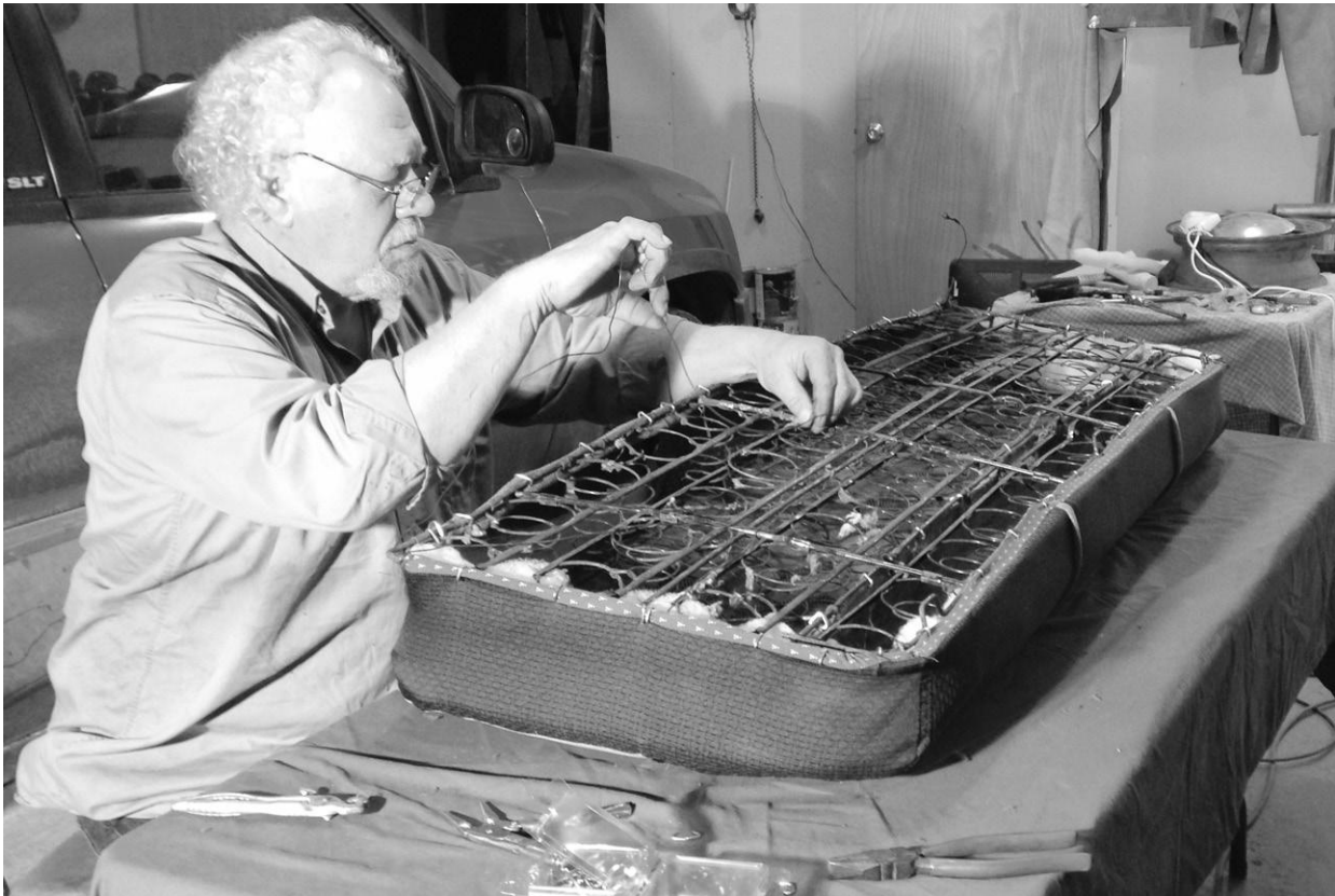
Dan Brand, works on the springs for the seat in the 1947 Frazer he restored. The car was a one owner vehicle, bought direct from the factory.
