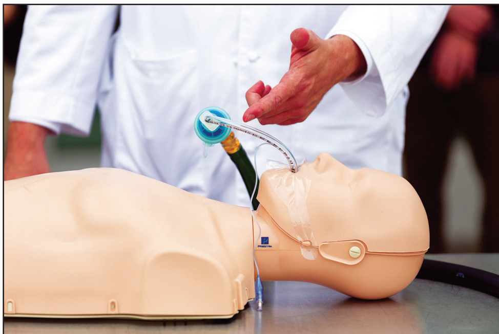
The ventilators were built from garden hose and other readily available parts. The ventilators are meant for use only if UMMC exhausts other ventilator options.
