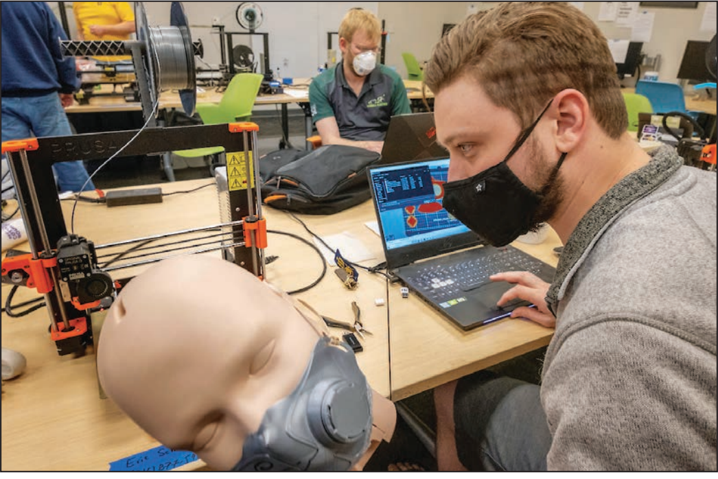
Eric Schneider, a senior aerospace engineering student at Missouri S&T, tests the fit of a prototype 3-D printed surgical mask on the head of a mannequin in the Kummer Student Design Center at S&T. In the background is Stephen Williams, an S&T mechanical engineering student. Photo by Tom Wagner/Missouri S&T.
