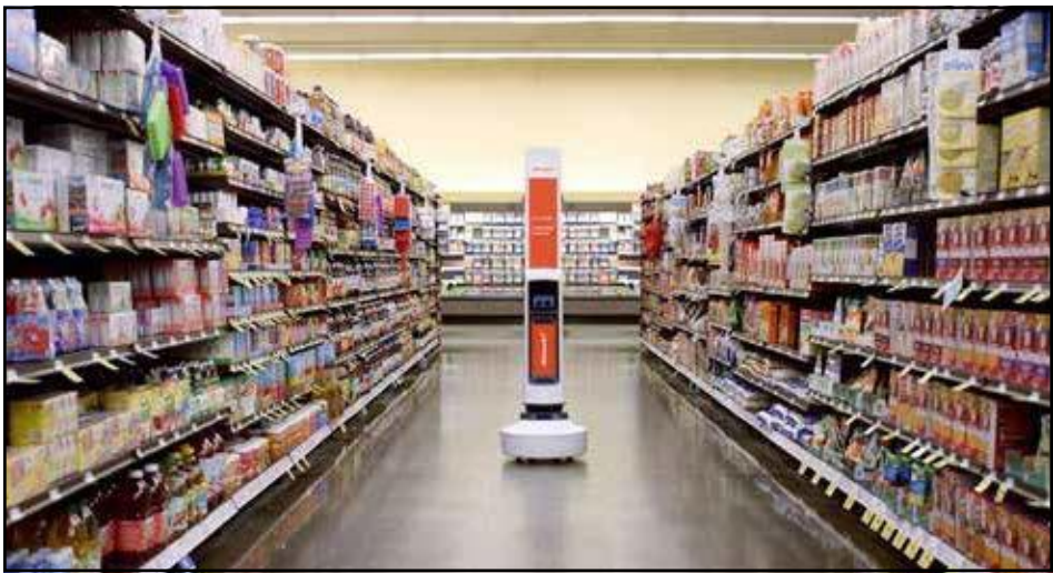
Simbe Robotics’ autonomous robot Tally, which traverses store aisles two to three times per day and autonomously capture inventory for approximately 35,000 products per store with each traversal.
