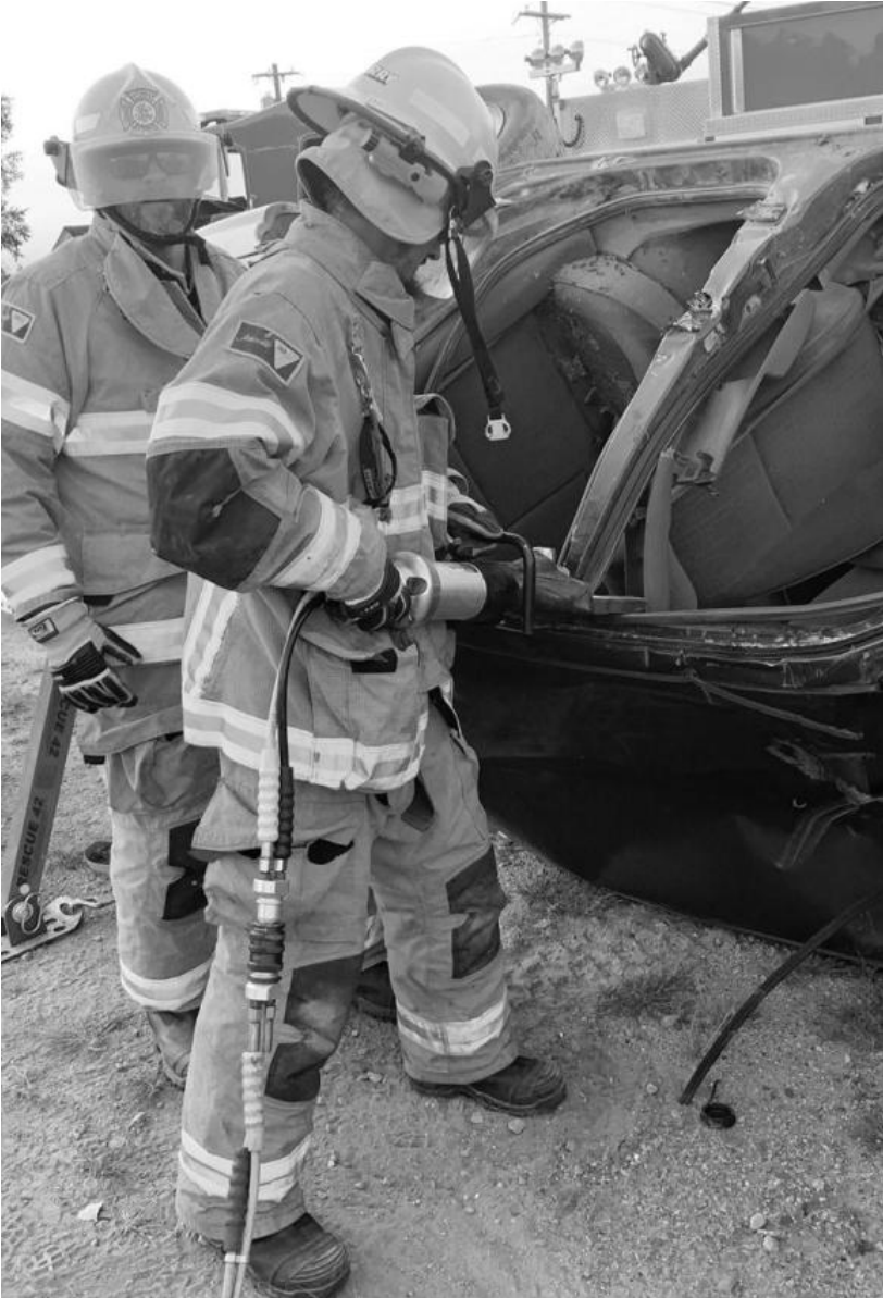
The Rothsay Fire Department recently conducted a fire practice devoted entirely to use of the “Jaws of Life”. This is a unique tool capable of using its jaws to cut through heavy metal. Or, when the hydraulically operated tool is used in reverse, it can force apart layers of steel. The tool is particularly effective in extricating victims from an automobile crash. In many cases the passenger or driver of the
