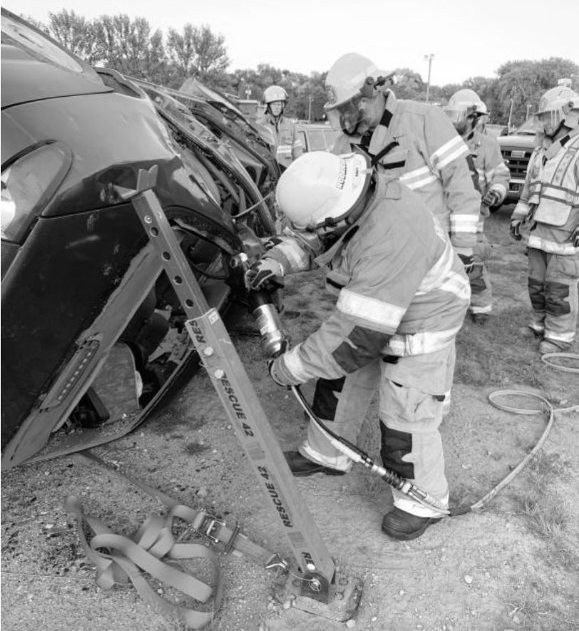
The Rothsay Fire Department recently conducted a fire practice devoted entirely to use of the “Jaws of Life”. This is a unique tool capable of using its jaws to cut through heavy metal. Or, when the hydraulically operated tool is used in reverse, it can force apart layers of steel. The tool is particularly effective in extricating victims from an automobile crash. In many cases the passenger or driver of the
