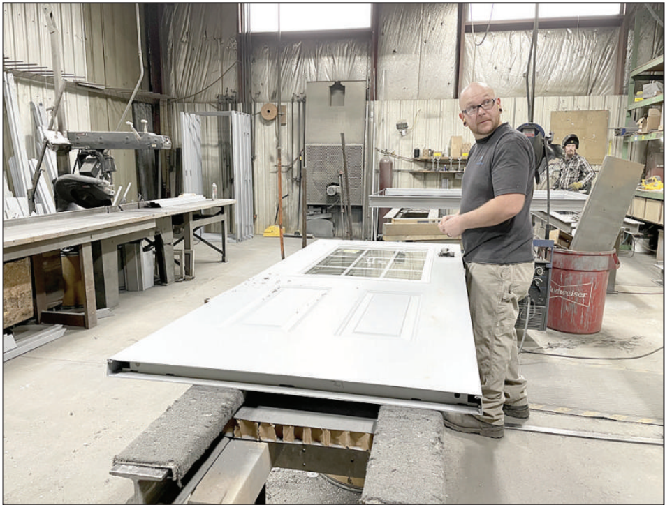
Jarad Franklin glances back as he works on installing a light kit in a hollow metal door.
