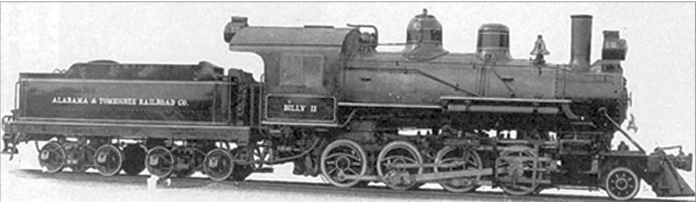
This Lima 2-8-0 (so named for the wheel configuration, 2 small front wheels, eight drive wheels and no rear trailers) was one of two rod engines operated by the Alabama & Tombigbee Railroad, Scotch Lumber Company's line. It was shipped to Fulton in November 1915 and named "Billy II." Billy Harrigan was the son of Scotch owner William D. Harrigan and would be an owner and lead the company in later years. It would be sidelined after the mill burned in 1930 and was sold in 1941 to a Montgomery gravel company where it worked for a time being, being scrapped. This is a Lima company photo and is attributed to the P. E. Percy Collection in the book "Logging Railroads of Alabama".
