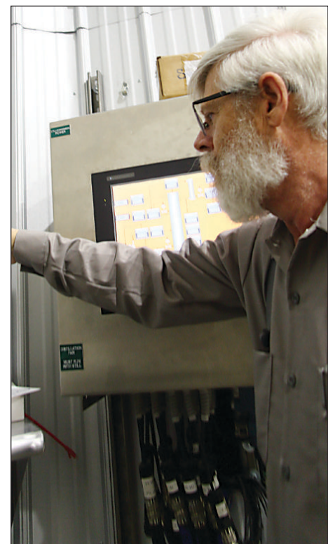
Dan Graham, checks the Brix on a sample pulled straight from the distillate flow last week. The measurement is used to calculate the finished alcohol content. Behind him is the display from the computer monitoring every minute detail of the process, temperatures, flow rates, pressures and other information.
