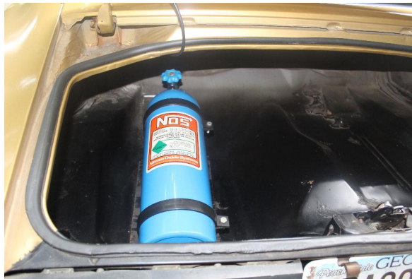
A little something extra, a 125 horse nitrous kit with tank in the trunk.
