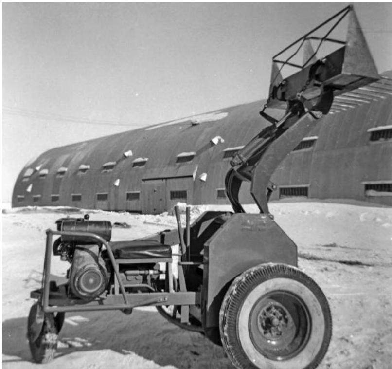
The Keller brothers’ three-wheeled loader, later refined and renamed the Bobcat® skid-steer loader.
