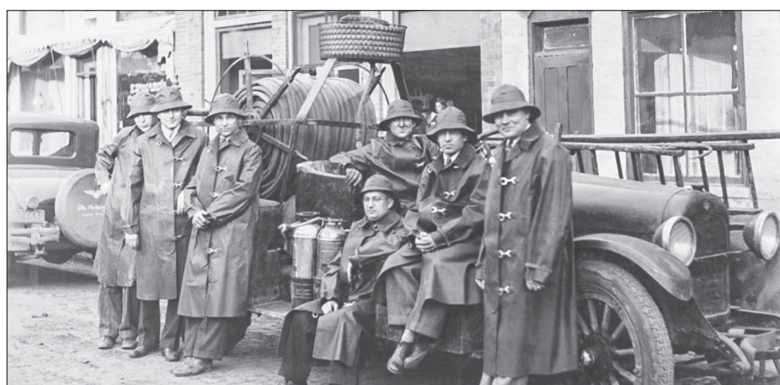
ARTHUR FIREMEN in front of their homemade fire truck that was built on a Nash car chassis circa 1925-30.
