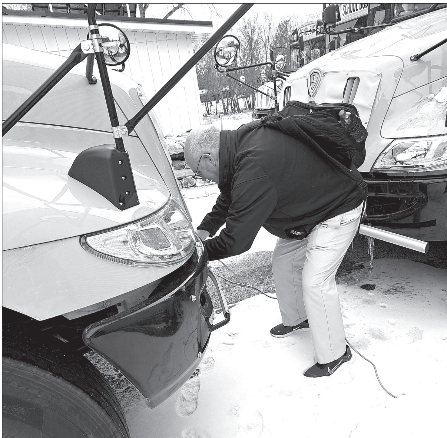
AFTER RETURNING from the game, Coach Sappenfield plugs in the bus to prevent the diesel from jelling. Photo by Tony Hooker.
