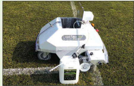
Shown in this photo is the GPS-guided Turf Tank robot used to mark the field for the Glen-Ed Soccer Club. (Rob Landers/Glen-Ed Soccer Club)
