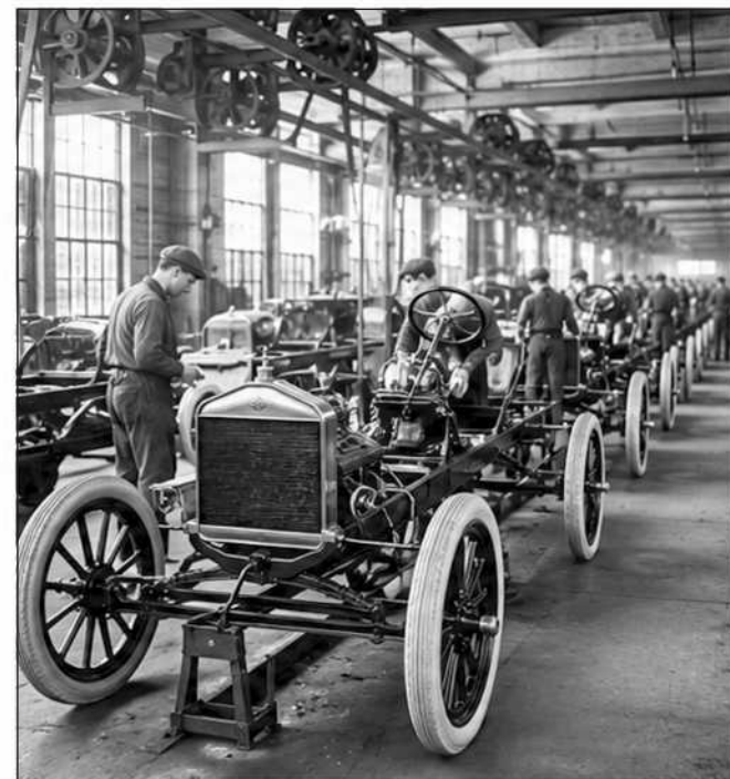
An assembly line at Ford Motor Co.'s Highland Park plant in 1913. The system introduced for the Model T helped speed production and make parts more widely available.
